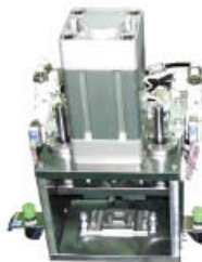
FORMING JIG FOR SUPPORT LINE
